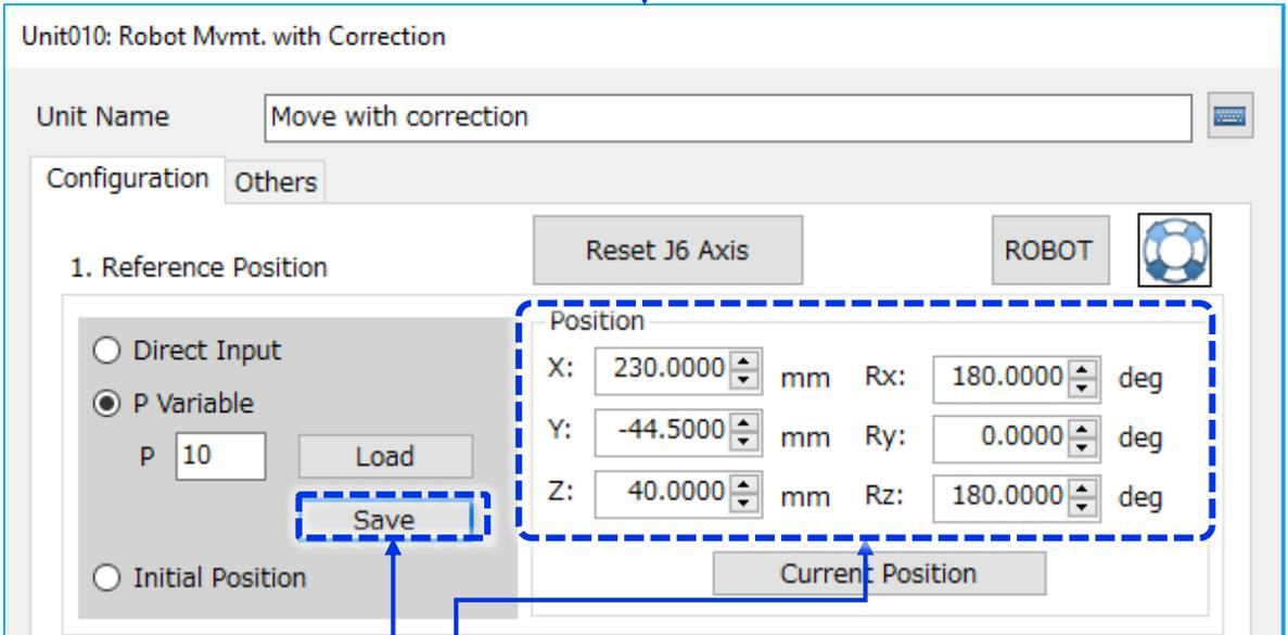
Enter the following coordinates accurately in the input fields for pick reference position setting.
