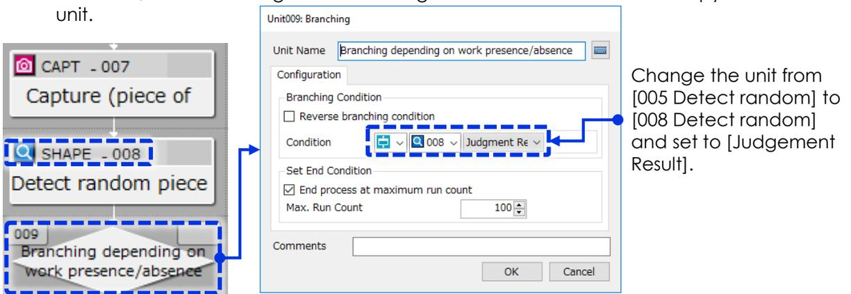
**3** Connect the "No" side of [009 Branching depending on work presence/absence] at the copy destination to [End].
