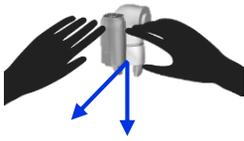
Move the hand in the same orientation as when it is actually performing the pick operation.
