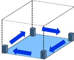
Move the arm to the lower four corners of the random pick area without changing the orientation of the hand, and confirm that no motion range errors occur.
