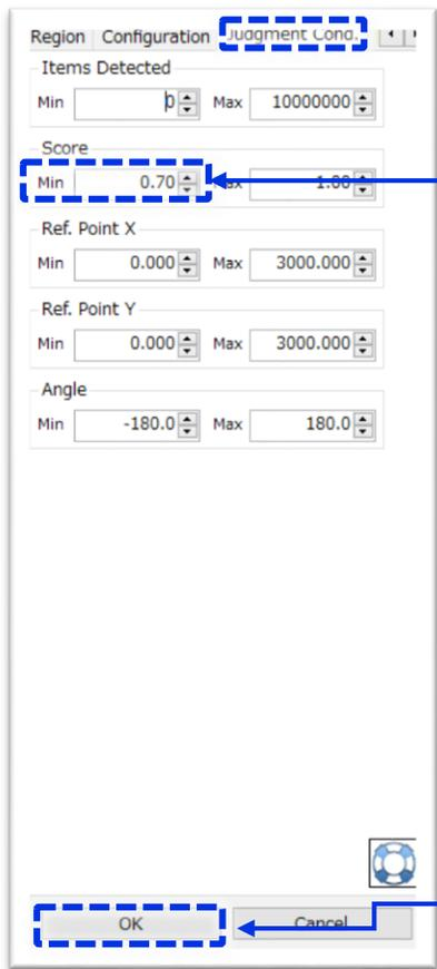
Adjust the minimum score (around 0.70) on the [Configuration] tab, and the minimum score (around 0.70) on the [Judgment Cond.] tab, to determine whether detected workpiece's position and angle is accurate.
