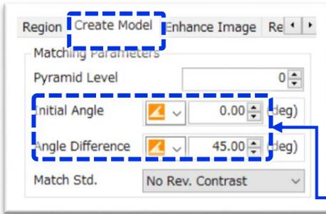
If the workpiece is symmetrical both left-right and up-down, registering  $180^\circ$  as shown below is sufficient.
