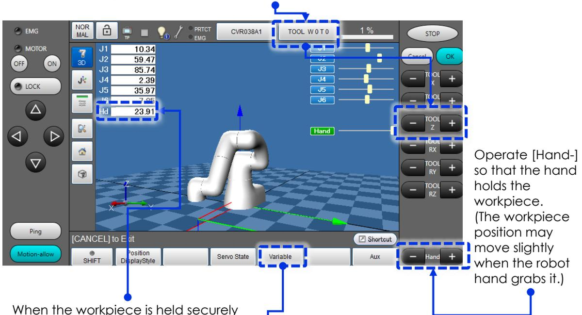
When the workpiece is held securely by the robot hand, make a note of the "Hd" value.
