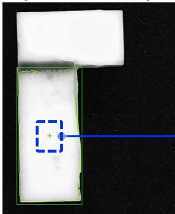
Model of the entire workpiece (The center position shifted toward the top right.)
