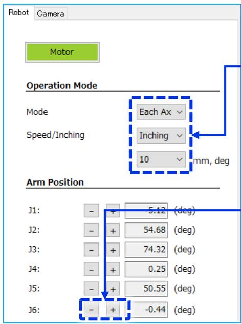
Set [Each Axis] to operate in J6 axis. Recommend to set [Inching] and move set amount by each mouse click. Select appropriate inching amount.
