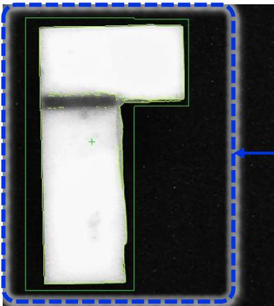
Using two rectangle regions, enclose the entire workpiece as L shape region.
