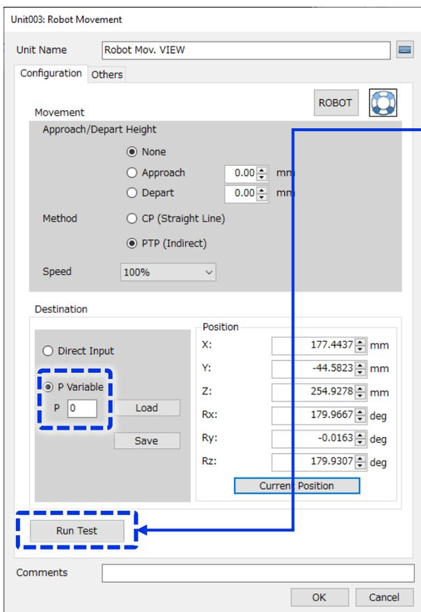
In this example, by clicking [Run Test], the robot arm moves to the P0 position (=image capture position).
