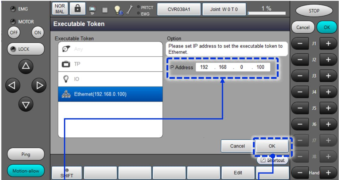
If the token is set to Ethernet, enter the IP address of the Vision Edition IPC and not the computer running Virtual TP unless they are running on the same PC hardware.
