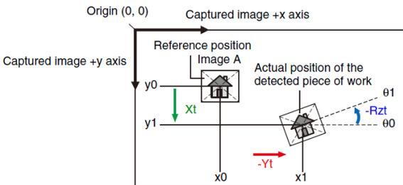
To calculate the displacement from Image A as shown in the left, vector adjustments below are required. (Assuming J6 is set to 0° at pick reference position and only Xt, Zt movement used to arrive to image capture position.)
