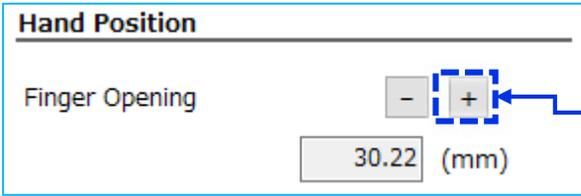
Carefully open the hand but making sure that workpiece position does not move. Then click [Close] to close Robot Control window.
