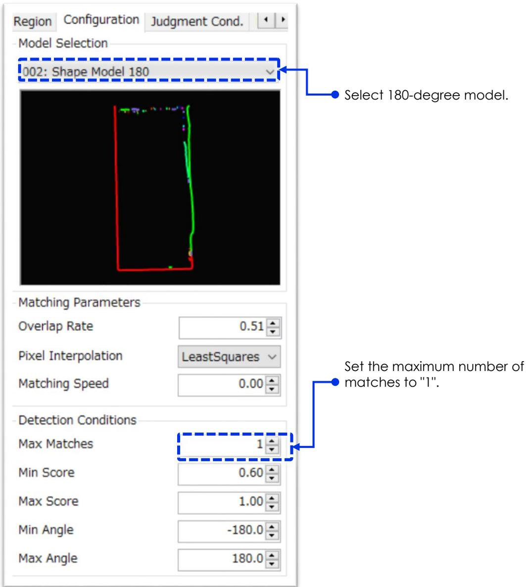
9 Click the [Manual Trigger] button at the top of the screen, and check if the workpiece is recognized correctly. Move the workpiece in a variety of angles to check for the accurate detection.
