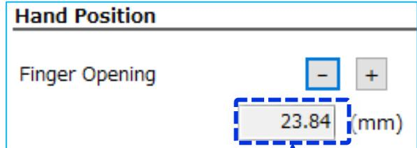
When the workpiece is grabbed, make a note of the finger opening of the hand.
