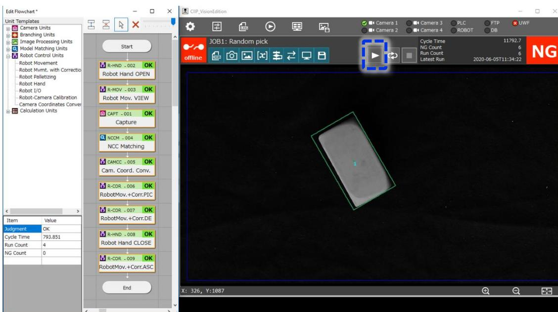
If the job runs correctly, the result for the flowchart operation units should be OK. In this example, the result displayed in the upper right corner is NG, but that is merely because of the default settings.
