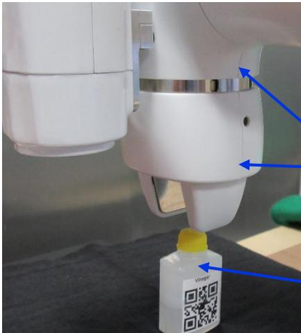
As J6 approaches 0°, these lines will align. When viewed from the front, the camera and hand will be in a straight line.
