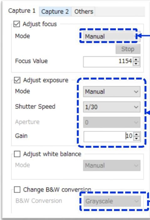
Tick box and set to [One-Shot AF] to align the focus position with the workpiece.
