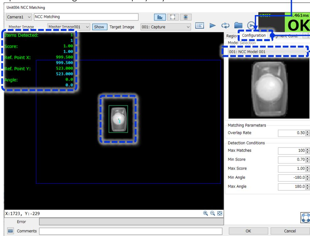
Change the position and angle of the workpiece in the pick region, then click [Trigger] to run detection tests.
