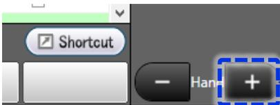
Click [Hand+] a few times to release the workpiece. Make sure to release the workpiece slowly so that it does not move.
