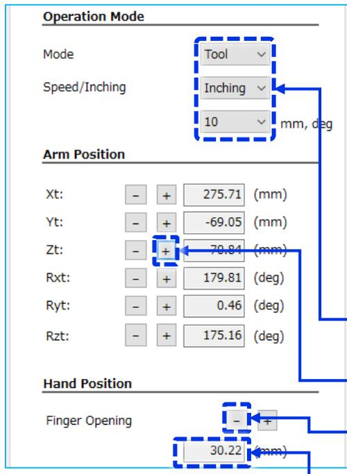
Place the workpiece to the position/angle so that lowered robot hand can correctly hold.
