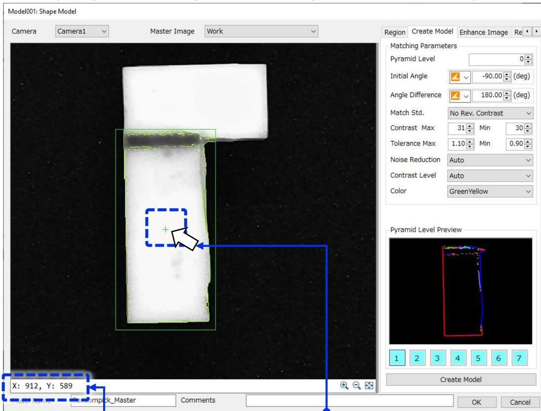
Move the mouse cursor to the center of the workpiece green cross, and make a note of the coordinates shown on the bottom left.
