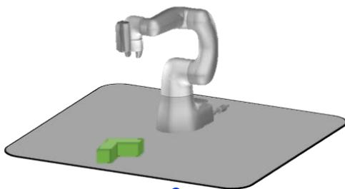
If picking is by 360-degree model based on entire shape, it may not be able to pick up always.
